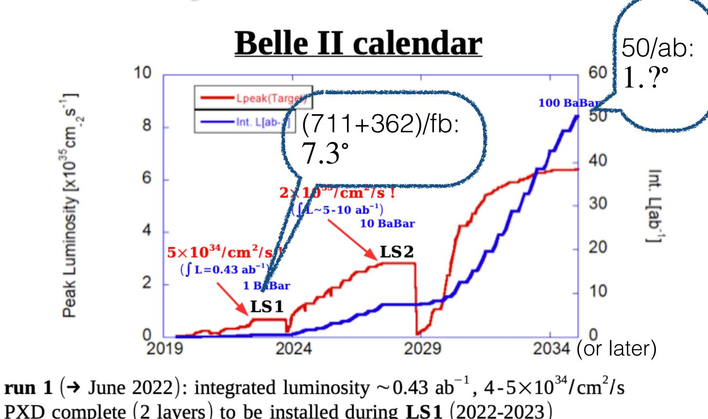
PXD complete (2 layers) to be installed during LS1 (2022-2023) (+beampipe + TOP PMTs) **run 2** ( $\rightarrow$  2027): integrated luminosity 5-10 ab<sup>-1</sup>, 2×10<sup>35</sup>/cm<sup>2</sup>/s
