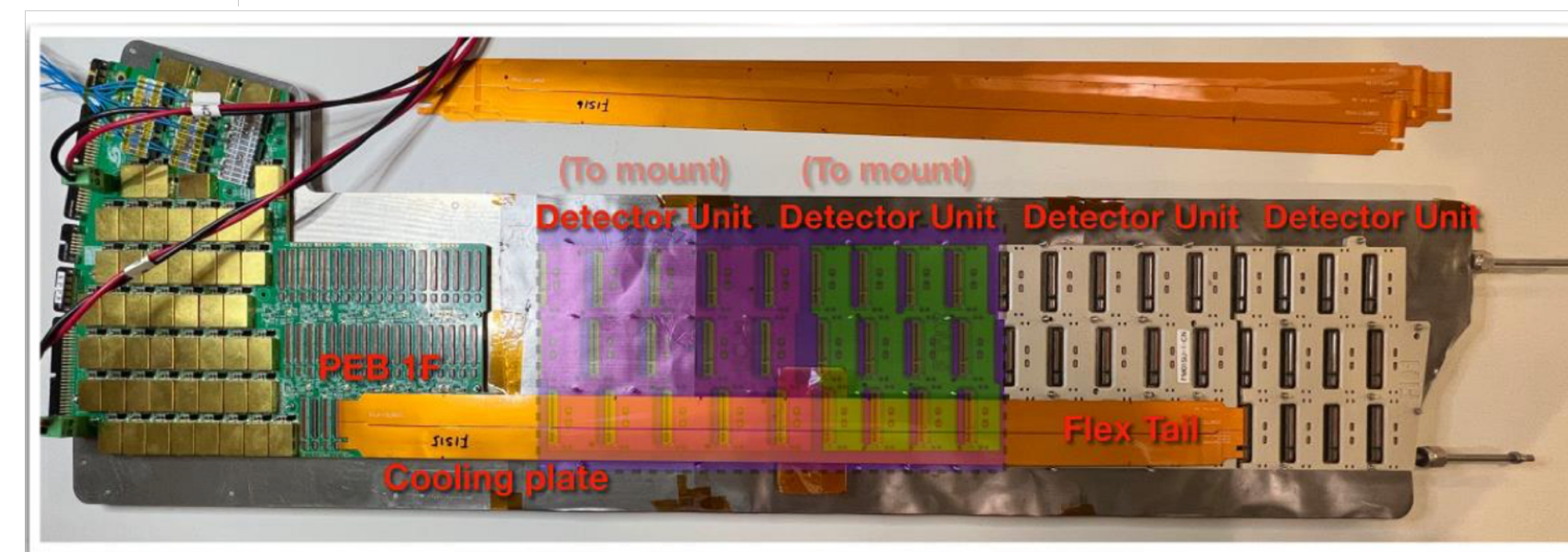
HV, LV, Cooling plate prototype Electronics : PEB 1F + flex tails + 54 modules mounted on 4 support units (detector unit)
