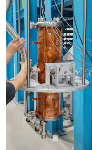
HWR010 Cu/Nb cavity on vertical test stand
