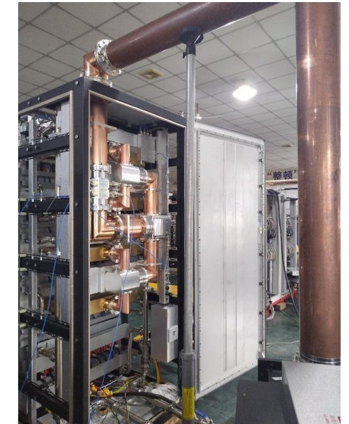
Measurements of 60 kW GaN rack with dummy load.
