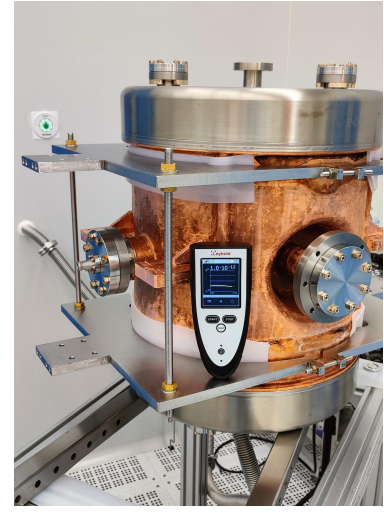
The assembled HWR040 CuNb cavity in clean room
