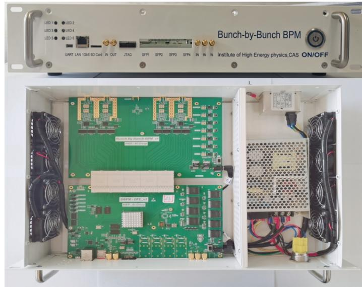
Bunch by bunch measurement and processor
