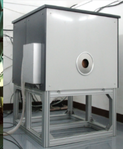
9MeV accelerator X-ray source
