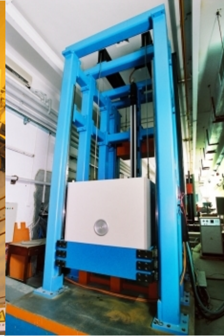
6MeV accelerator X-ray source
