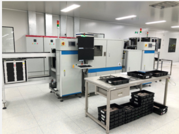
Computed Laminography for IGBT testing
