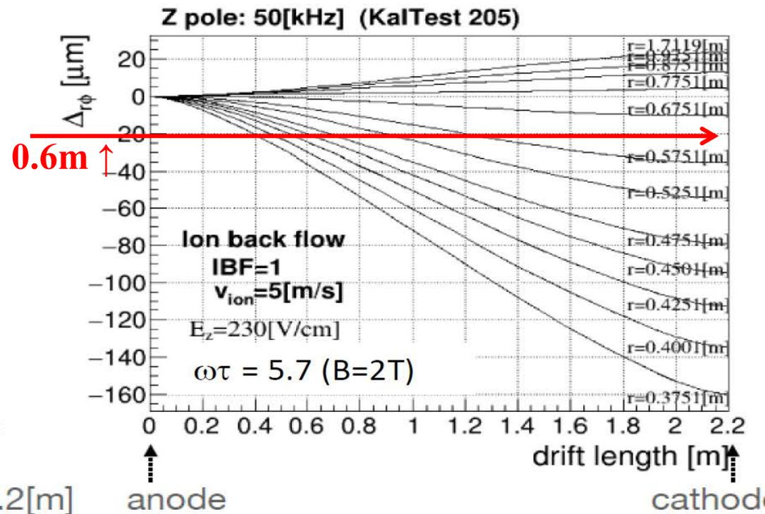
Maximum distortion  $\sim 160$  [ $\mu$ m] at the innermost region for hadronic Z rate of 50 [kHz]
