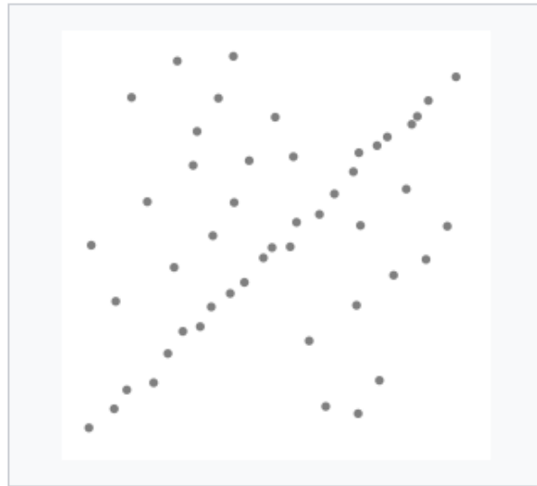
A data set with many outliers for which a line has to be fitted.
