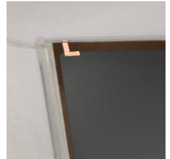
HV link applied
