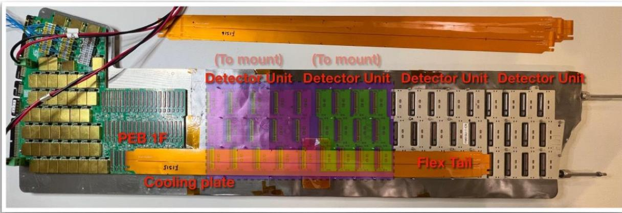
HV, LV, Cooling plate prototype
