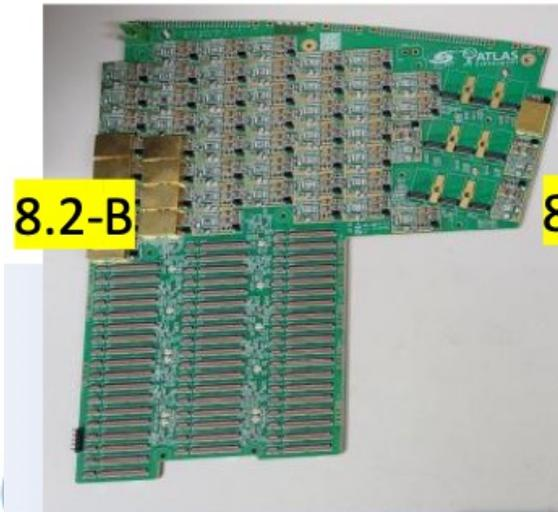
High voltage power supply prototype
