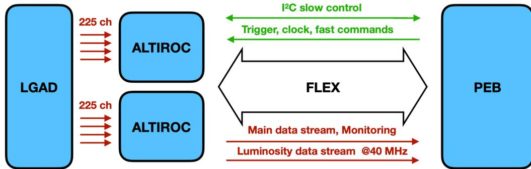
Modular Peripheral Electronics Boards prototype
