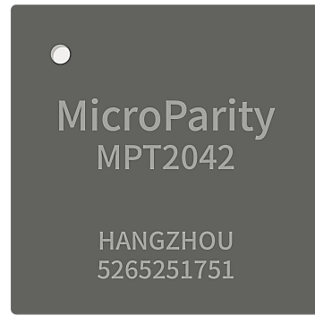
MPT2042 5mm*5mm QFN32 package
