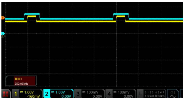
TDC injection signal f = 250kHz T = 4us
