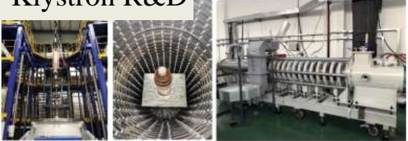
Klystron No. 1 Efficiency 65% (2020)
