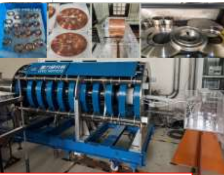
Klystron No. 3 (MBI) Efficiency 80.5% To be completed in 2024
