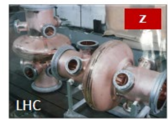
400 MHz 1-cell cavities Nb/Cu, 4.5 K
