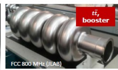
800 MHz 5-cell cavities Bulk Nb, 2 K
