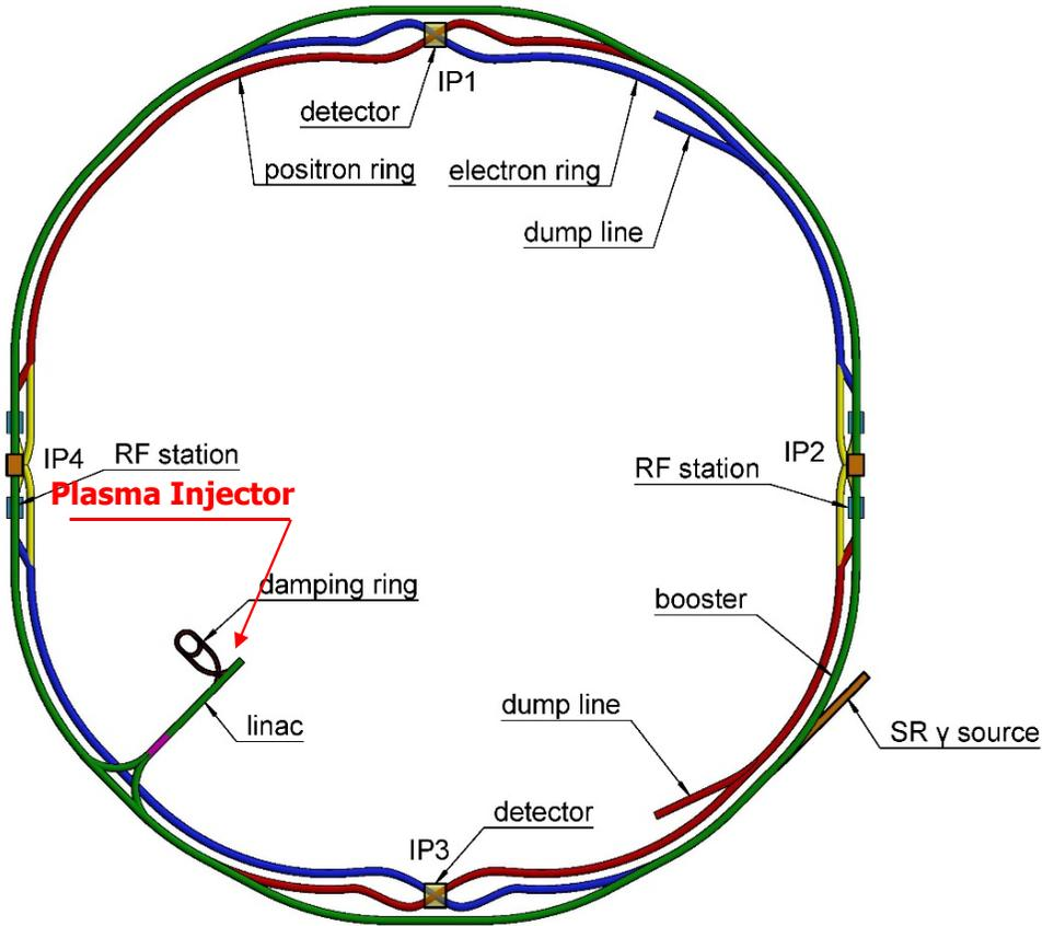
10 GeV e-/e+ beam in a 100 km ring
