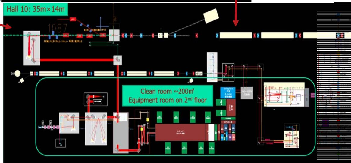
2.5 GeV e-/e+ beamline + PW-level high performance laser system
