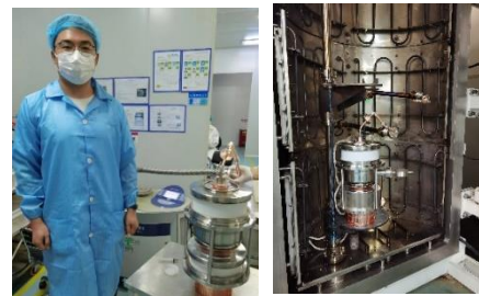
Degassing furnace evacuation
