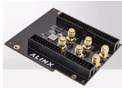
FMC daughter cards used for tuner control
