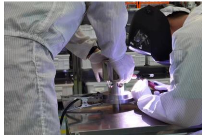
Welding of the cathode and focusing electrode of the electron gun
