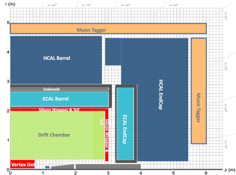
ALLEGRO Detector Concept for FCC-ee
