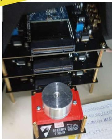
$^{55}\text{Fe}$  source with Aluminum collimator
