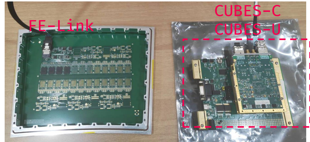
Pixelated TPC module for Beam test
