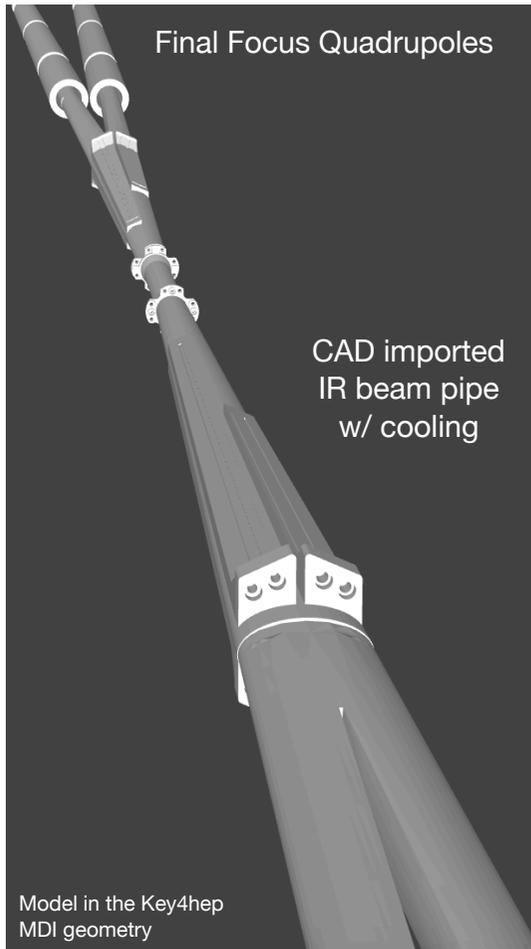
**Engineered CAD model** of AlBeMet162 beam pipe imported in **Key4hep**.
