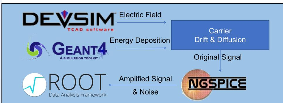
Figure 1. Simulation work flow by RASER [1].
