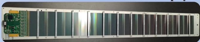
Fig. 2: Detector unit(ladder) of AMSL0
