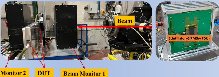
Fig. 3: Photo of beam test setup
