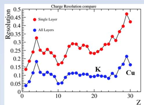
Charge resolution of single layer and telescope
