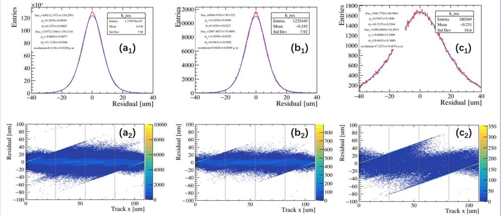
Fig. 6: Residual distribution and residual of in-strip hit position distribution of different regions: (a<sub>1</sub>)(a<sub>2</sub>) normal region; (b<sub>1</sub>)(b<sub>2</sub>) bias resistor region; (c<sub>1</sub>)(c<sub>2</sub>) no intermediate strip region.
