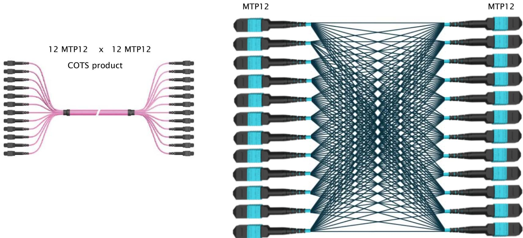
A 60 MUX nodes to 60 GEP nodes full mesh optical fibre exchange can be constructed from above COTS product easily.
