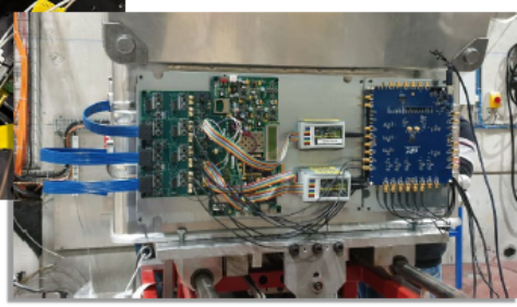
External view of the setup, displaying FPGA and mezzanine (green boards), IIC interface (white boxes) and clock generator (blu board).
