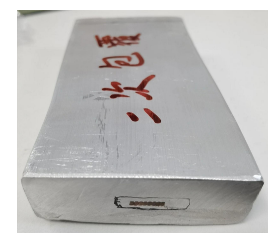
Dummy cable 56*22mm Aluminium alloy+ copper4.7mm*15mm
