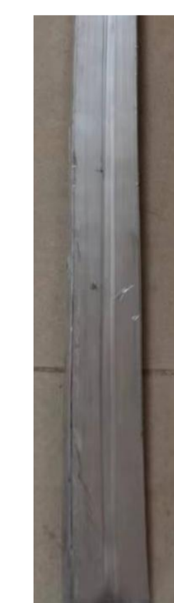
first co-extrusion pure Aluminum +Rutherford cable10*33mm
