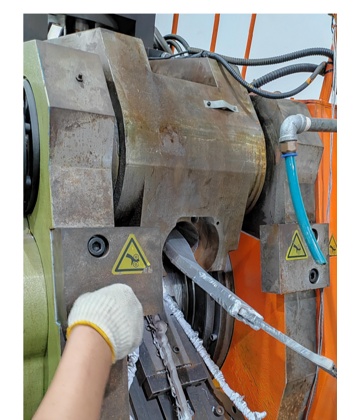
second co-extrusion 6061 Alloy+cable(failed)
