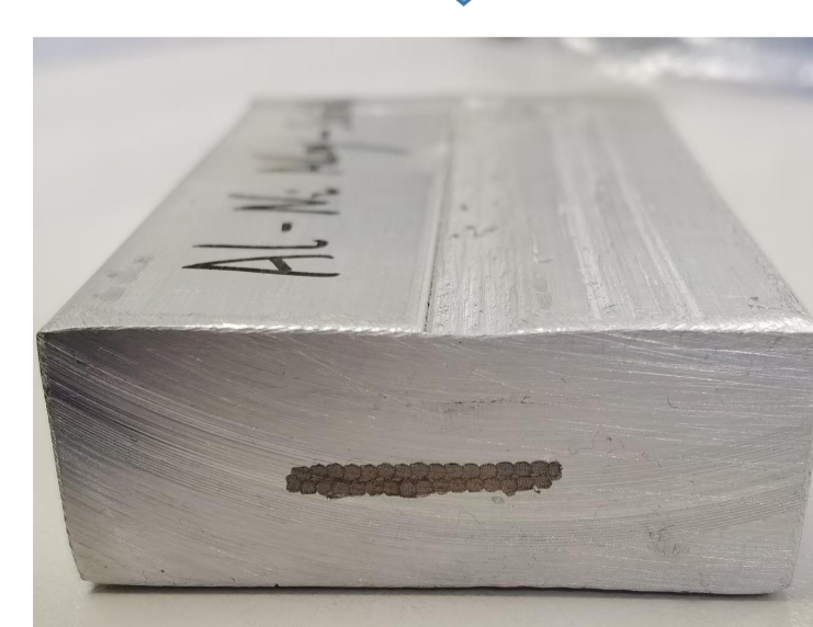
first co-extrusion Al-Ni-Be stabilizer +Rutherford cable 56mm*22mm
