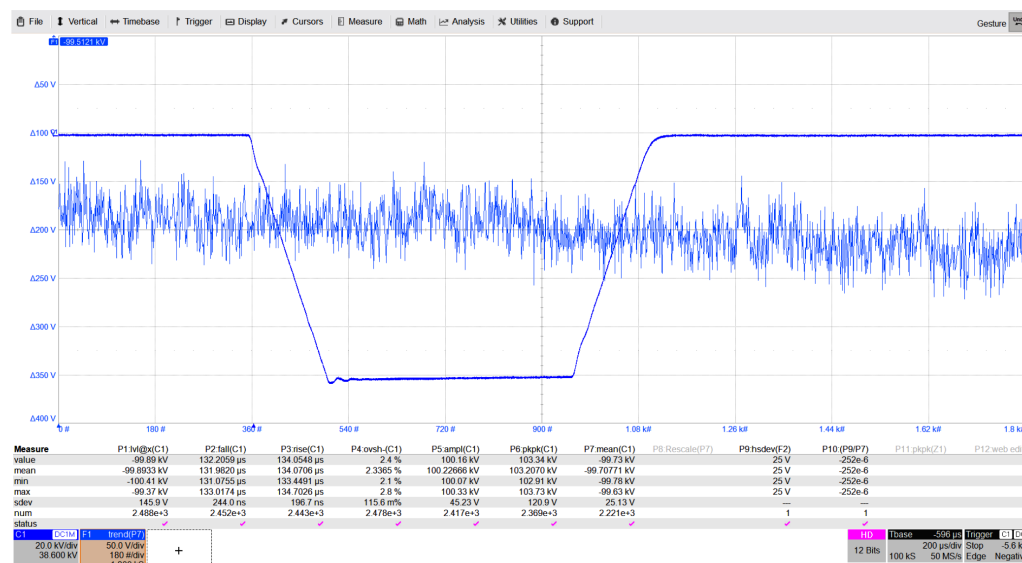
Pulse high voltage output (100kV/16A, max 200Hz)
