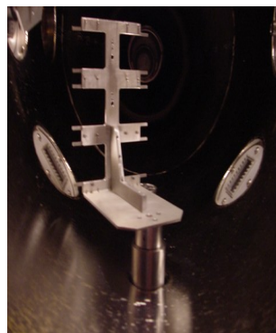
Very thin carbon strip target-20um x 25 nm
