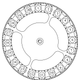
Rotating target holder. r_1 :124.1 mm, r_2 :145 mm
