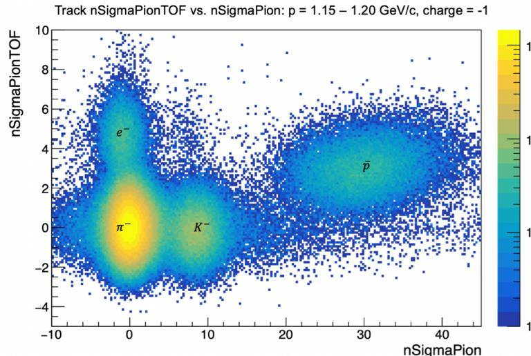
$$n_\sigma(\pi) = \frac{1}{\sigma_{dE/dx}} \ln \left( \frac{dE/dx_{\text{meas}}}{dE/dx_{\pi, \text{calc}}} \right)$$
