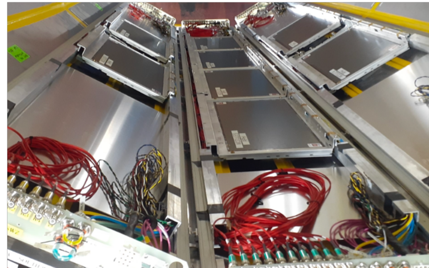
Micromegas detector Partial coverage outside of TPC 100 \mu\text{m} position resolution
