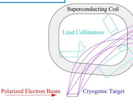
3.0 GeV electron beam, 40 uA 20 cm long LH2 target
