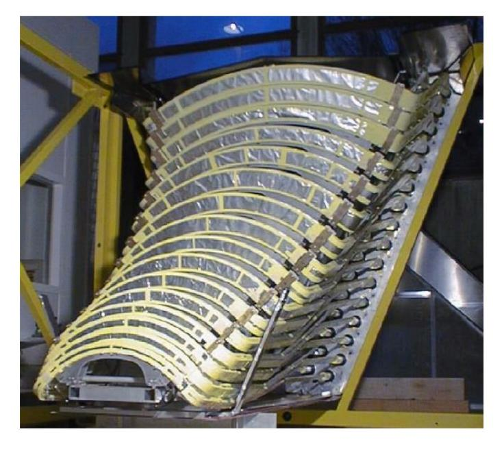
One "octant" of scintillators, to be positioned in the focal plane of the spectrometer. Each scintillator has two PMTs, one on each end. There are two layers of scintillators; a coincidence of both layers was required, to reduce backgrounds.
