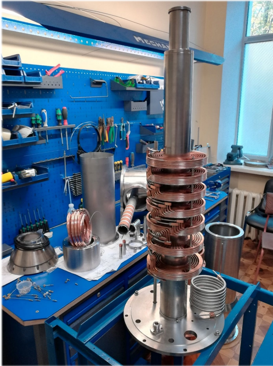
Parts of the dilution refrigerator during its manufacture at JINR (2018)
