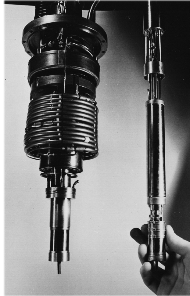
Dilution stage and sample container of the first Frozen Spin Target at JINR
