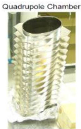
Figure 1a. One section of vacuum chamber set on a steel plate with the same curvature as the bending magnet.
