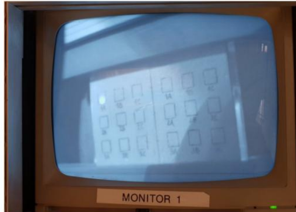
Monitor picture in MaMi control room: Beam spot on fluorescent screen in front of quartz samples
