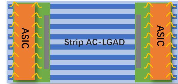
LGAD based strip silicon sensor prototype by IHEP
