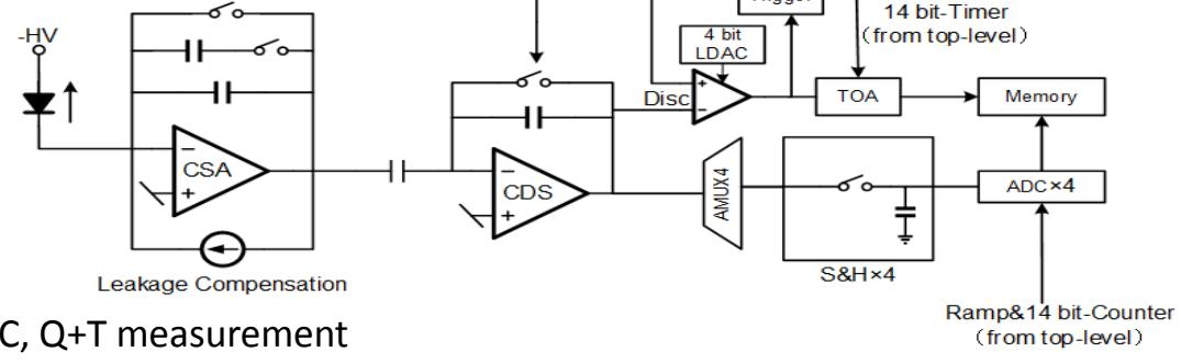
128 chn ASIC, Q+T measurement
