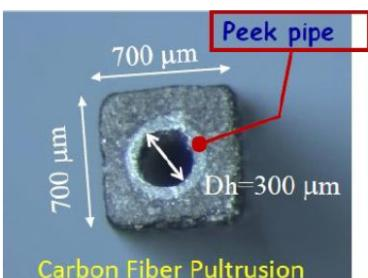
Alternatively, Lund is exploring micro channel cooling together with Pisa. These consists of pipes with Ø 300 µm in carbon fiber tubes.
