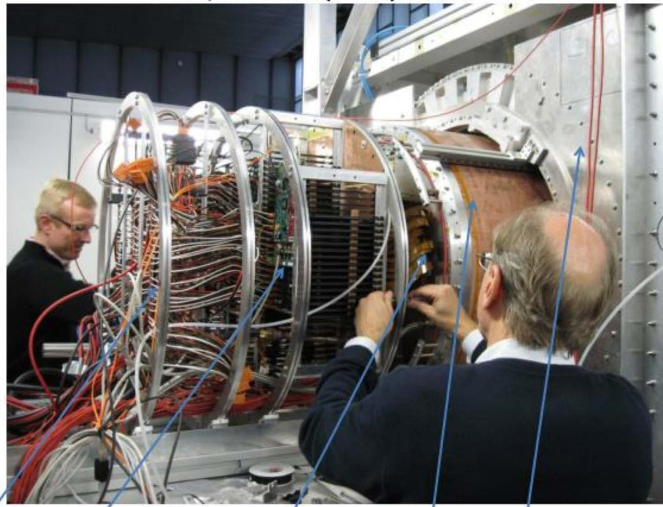
Low voltage    Front End Electronics    Kapton cables    TPC    Magnet
