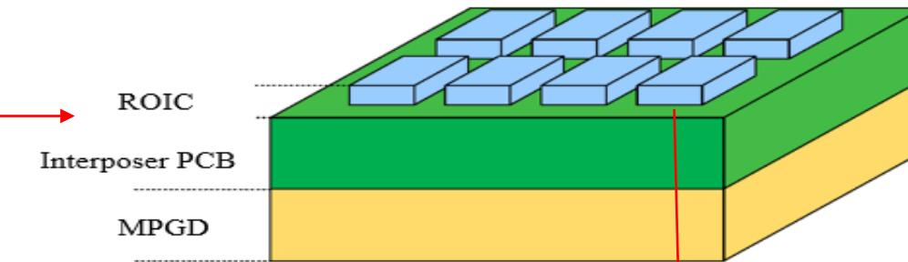
An integrated board with ASIC & MPGD, N(now 4) for a module
