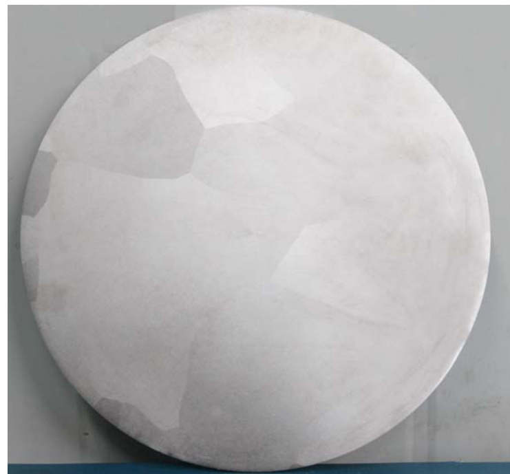
cross section of RRR Nb ingot
