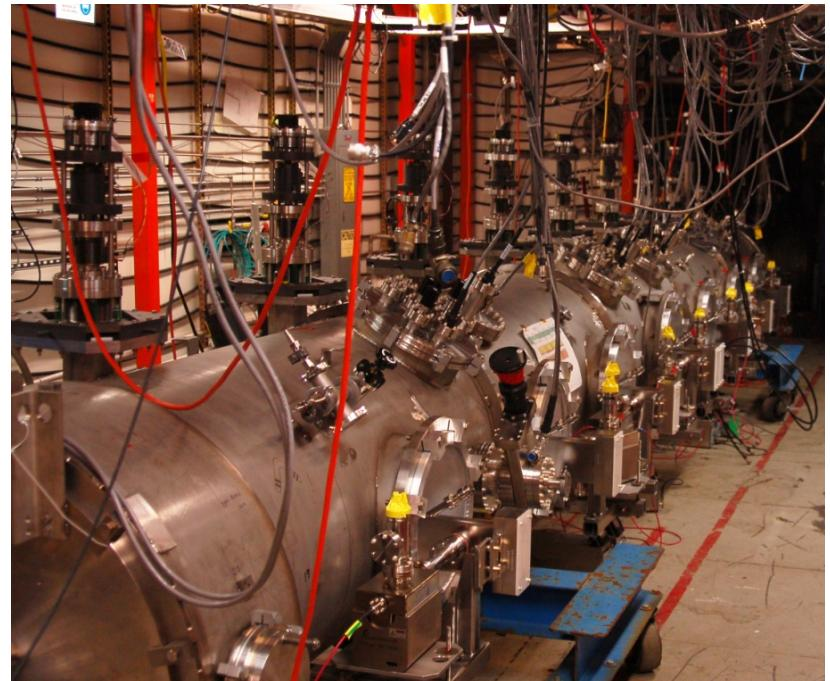
Cryomodule Assembly at JLab
