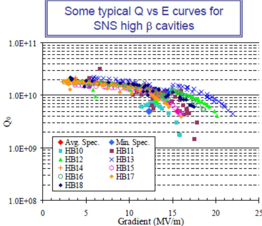
A predominant limitation of both medium- and high- $\beta$  cavities was unpredictable stray electron loading due to multipacting/field emission
