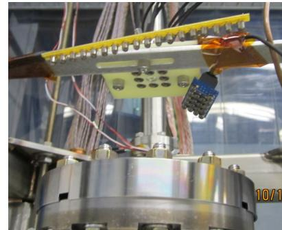
8 – Hamamatsu S1223 Diodes (provided by KEK STF) mounted above 9-cell cavity RI23
