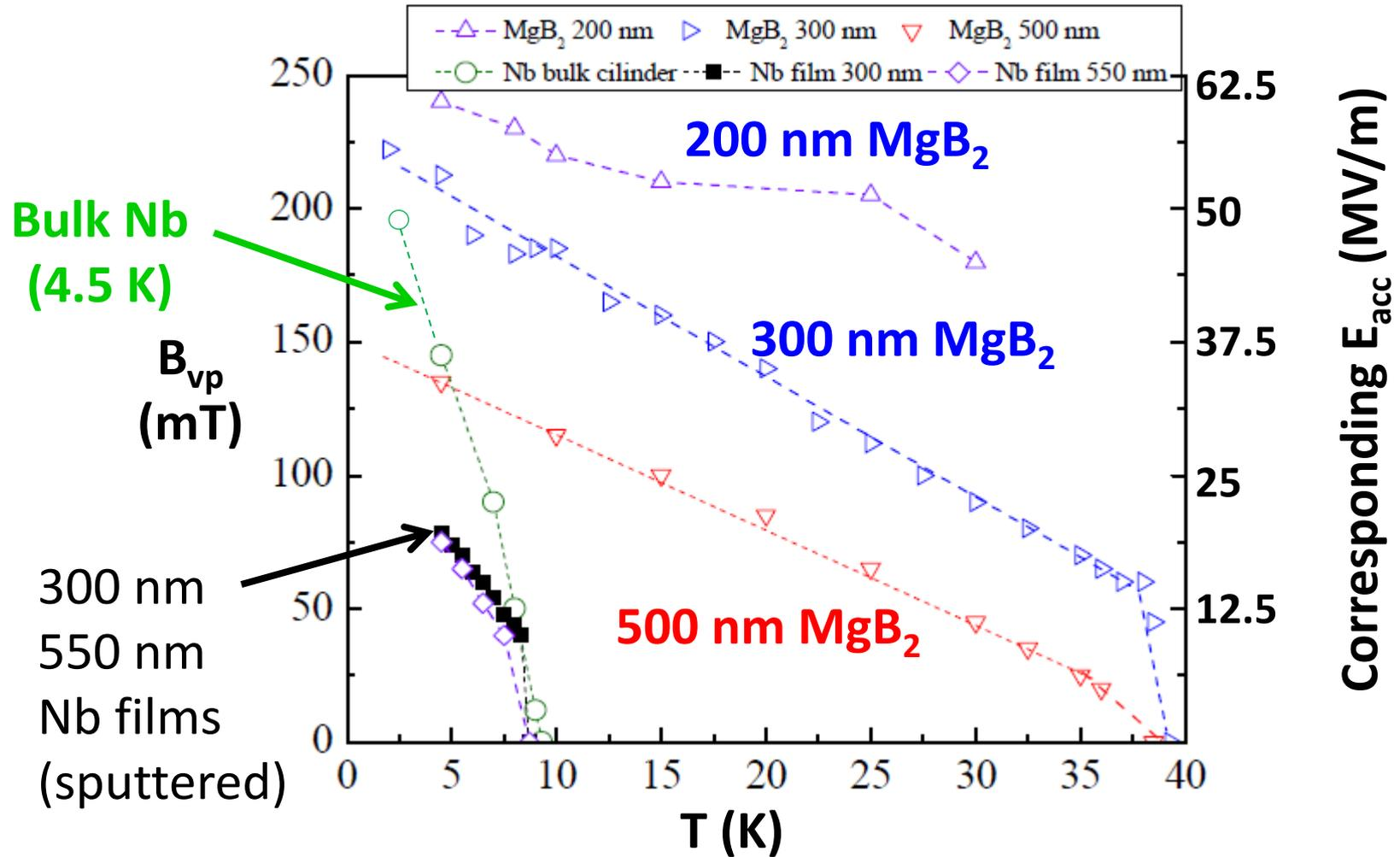
Measured  $B_{vp}$  were higher than expected  $B_{c1}$  ( $\lambda=110$  nm,  $\xi=6$  nm)
