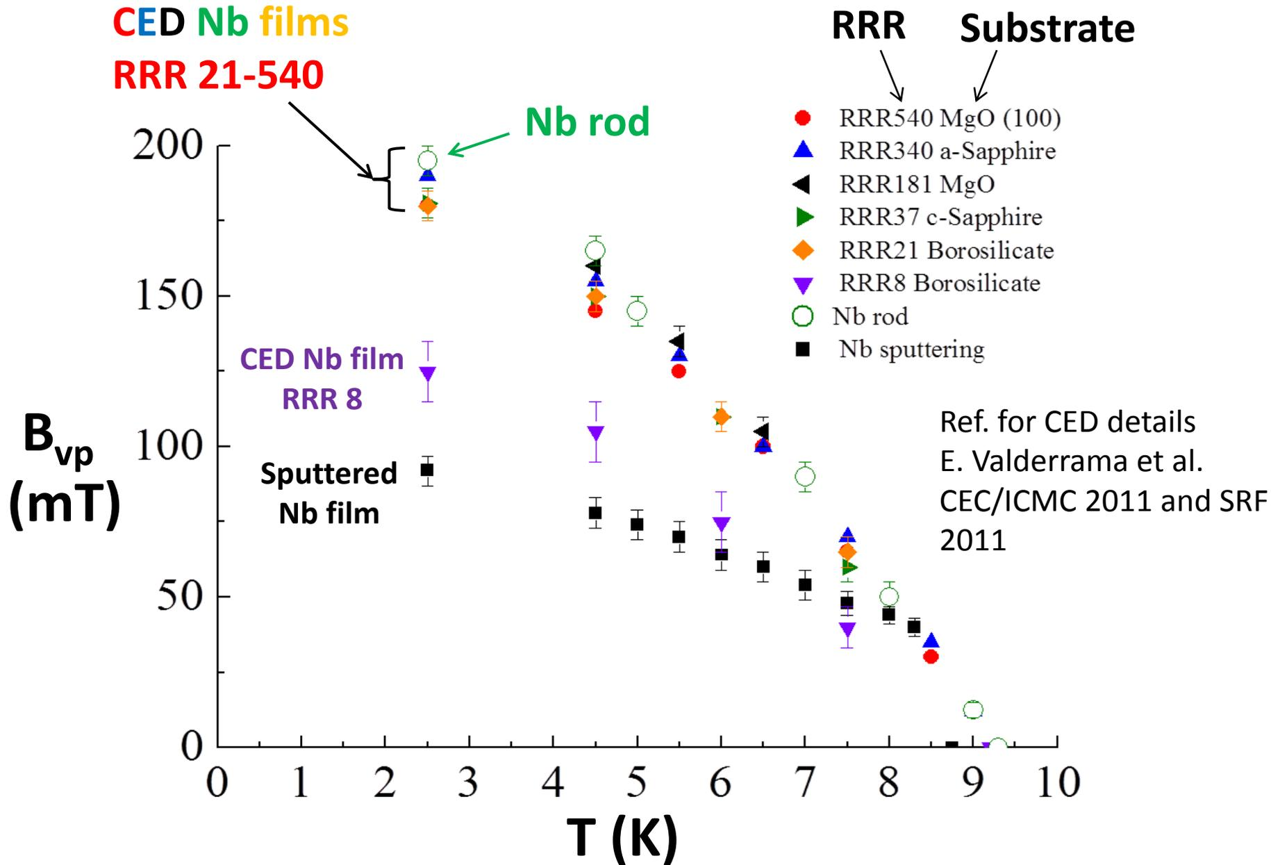
CED Nb on Cu at 300 °C has also shown  $B_{vp} \sim 170$  mT at 2.5 K so far.
