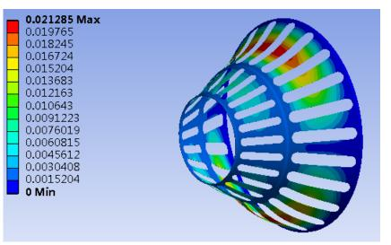
Deformation mm - under full load
