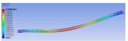
CFRP truss vertically supported: 0.04 mm
