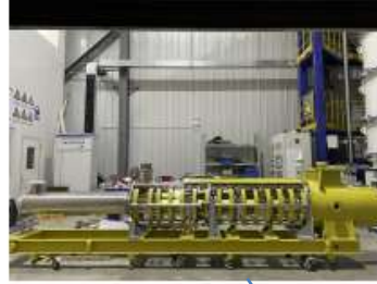
Klystron No. 2 Efficiency 77% (2021)
