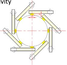
Sensor: R 12.5 mm, 148 W/m.k, 14.8x260x0.05 mm Beam pipe (beryllium): R 10.7 mm, 16 °C
