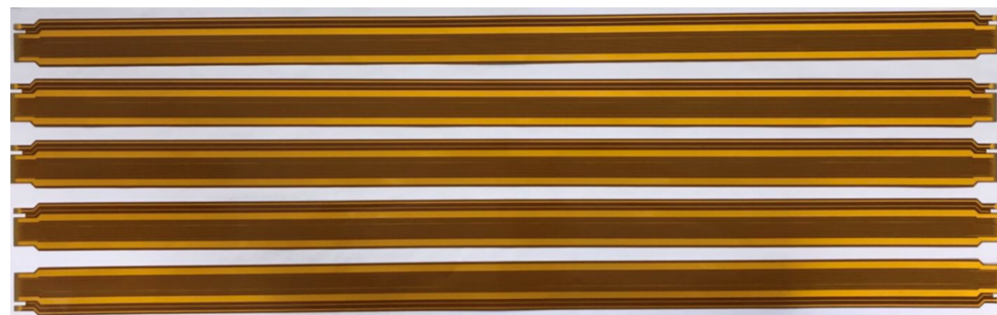
Long Flex tail prototype (75cm)
