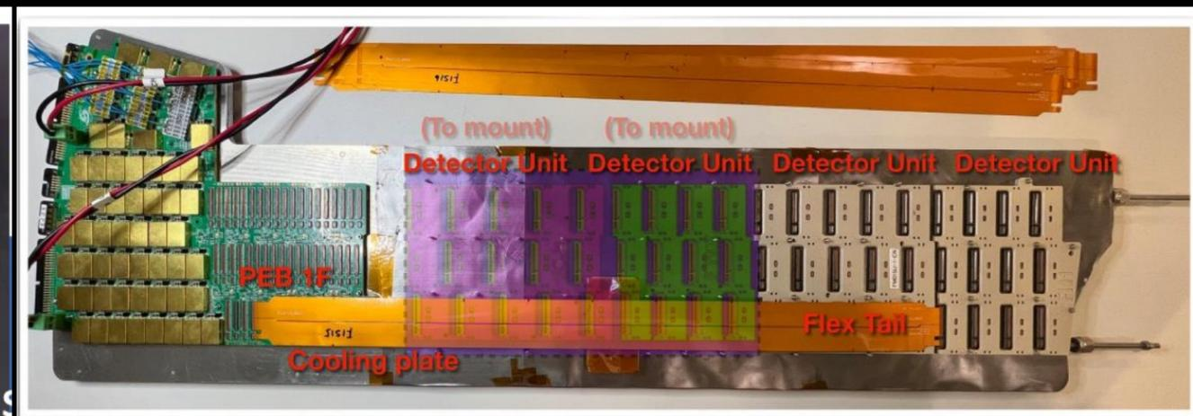
HV, LV, Cooling plate prototype
