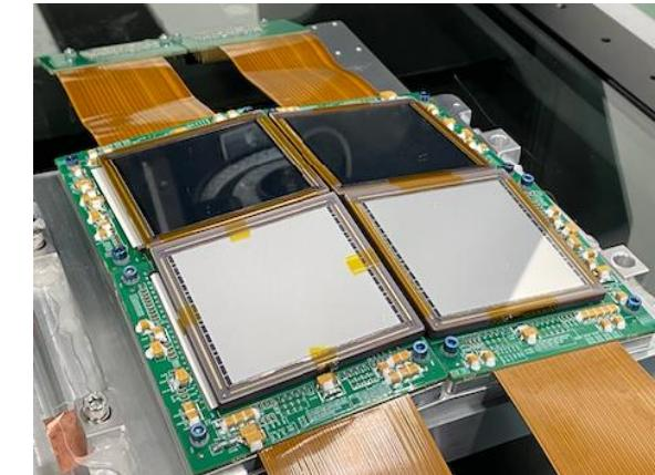
**BI CMOS sensors optimised for X-ray**
