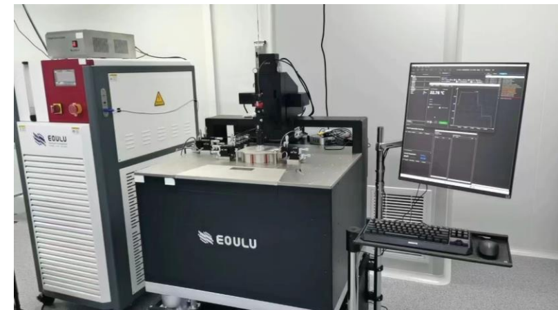
Semi-auto probe station for production QC
