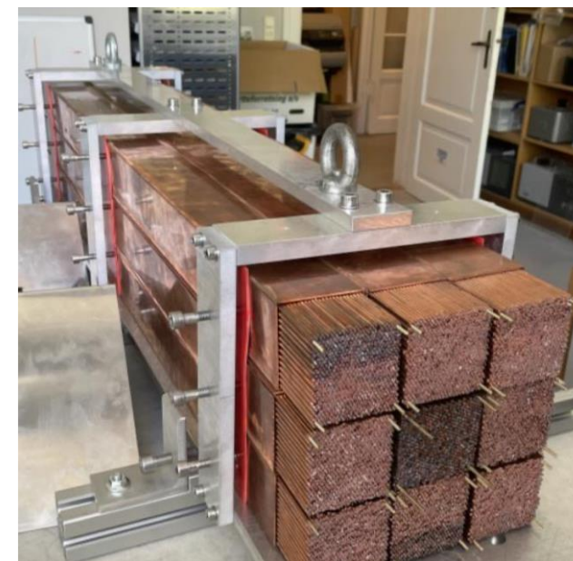
FoCal-H prototype, 9 \times (6.5 \times 6.5 \times 110\text{ cm}^3)
