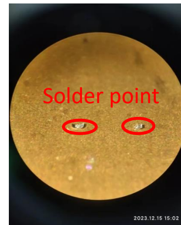
Pull test with DAGE4000
