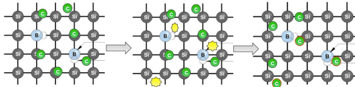
Irradiation Hardness Reinforcement by Carbon Doping:
