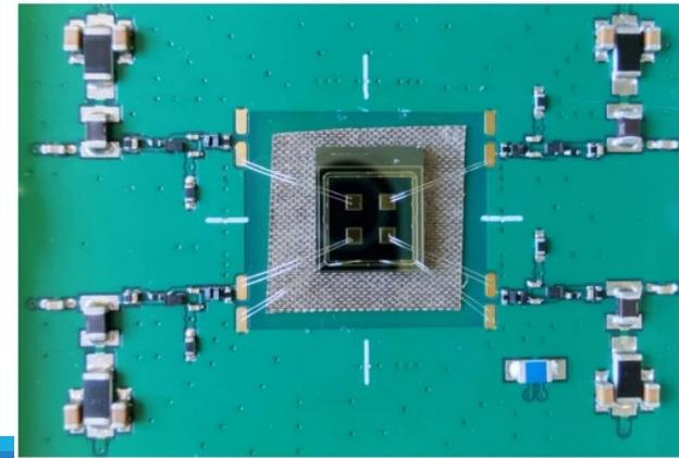
Position reconstruction, spatial resolution and timing performance of AC-LGAD be calculated based on the results from 4 pads.
