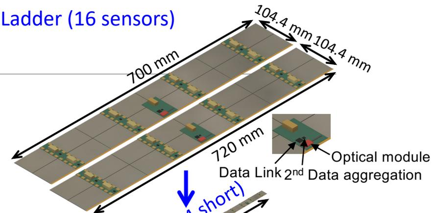
■ CEPC outer silicon tracker (OTK) utilizes AC-LGAD (Low Gain Avalanche Detector) developed by IHEP-IME:
