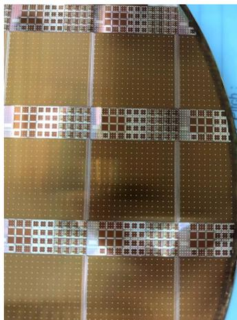
Altiroc wafer with ball for bump bonding
