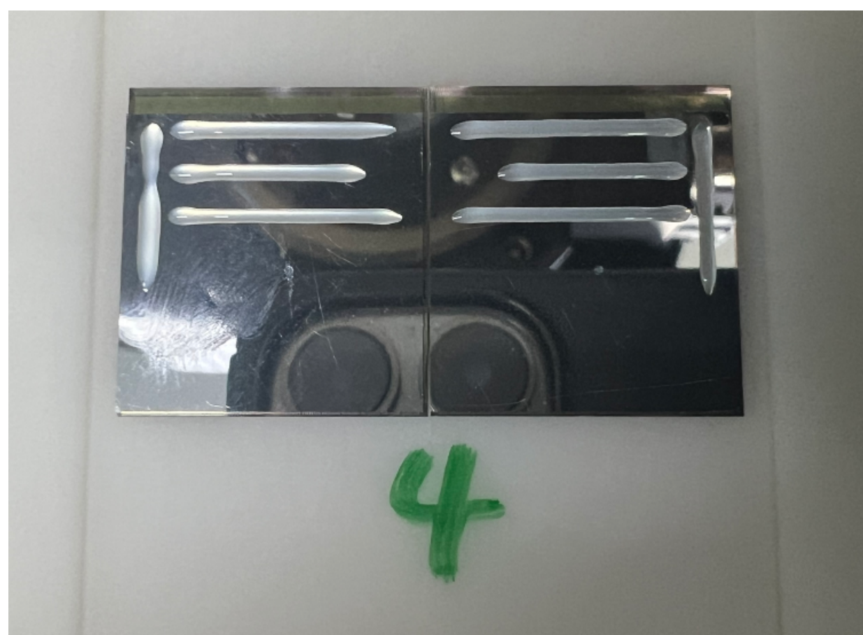
④ glue dots based on pre-defined weight and shape
