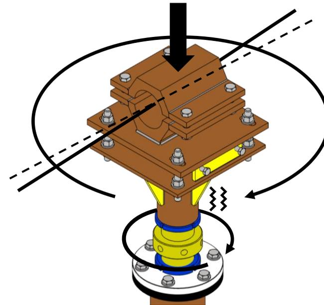
**Uncontrolled movement in the horizontal direction**
