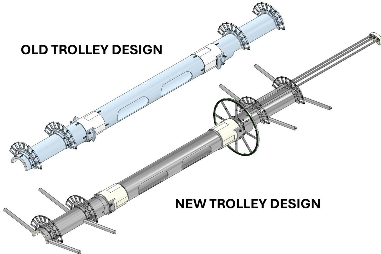
The old insertion trolley was **prone to bending** at the PTFE joints between aluminum pipe sections
