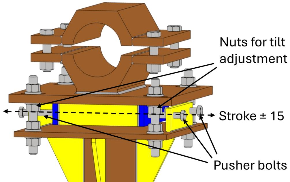
**Unlocking the nuts** to adjust tilt or horizontal position leads to **uncontrolled movement of the rail in the vertical direction**
