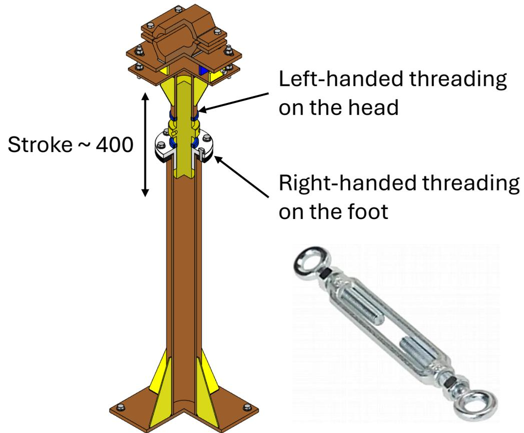
When **adjusting the height** under load, friction may transfer torque to the head
