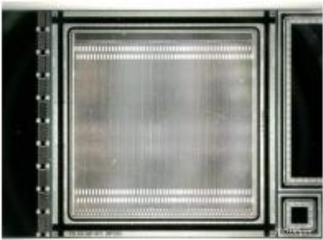
Silicon strip ITk mini sensor(left) and cross section(right)
